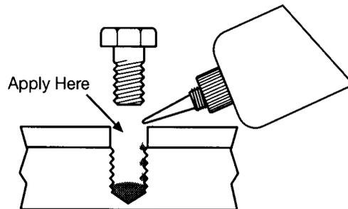
6. Assemble and tighten as usual. When tightening to established torque values, torque compensation is not required.
